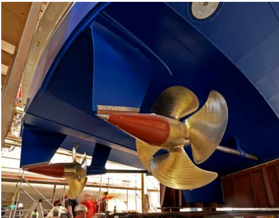
Launching of Nilo: the Servogear Controllable-Pitch Propellers
